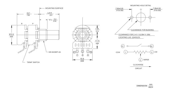
**270X-057X** Metal Shaft, Bushing Mount, Printed Circuit "X" Type Terminals, Rotary 057 Switch
